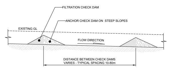
TYPICAL TRACKSIDE SWALE - LONG SECTION
