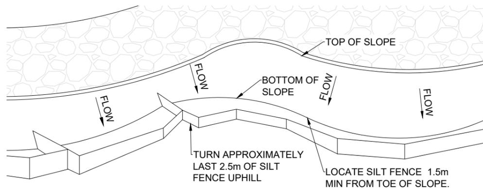
**TYPICAL SILT FENCE BOTTOM OF SLOPE**
